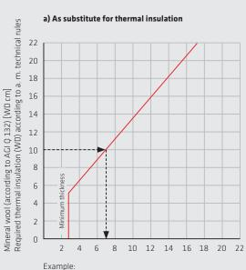
Required thermal insulation (WD) with mineral wool (according to AGI Q 132) according to manufacturer instruction: 10 cm
